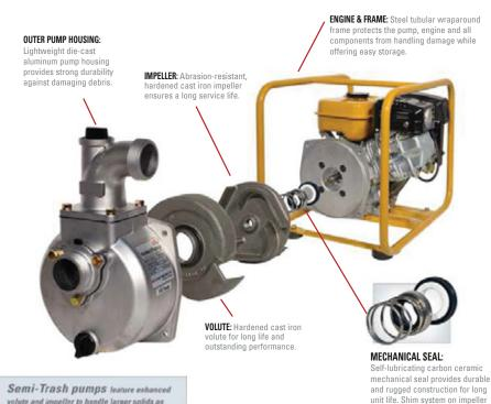
Semi-Trash pumps leature enhanced volute and impeller to handle larger solids as well as the silicon carbide seal system to ensure durability in challenging applications.
